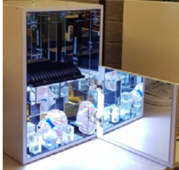
Figure 9: Sample do-it-yourself photobleaching cabinet with LED lamp and mirrors.
