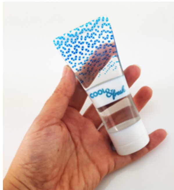
Figure 2: Soap tube prototype printed with VeroUltraClear.
